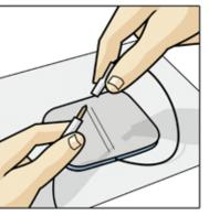
While disconnecting or inserting pin, hold the pin connector
